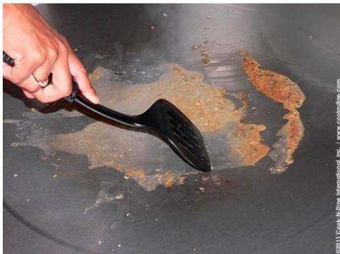
To eliminate the last traces (if any) the surface has to be **COLD**. Use a non-scratch nylon-mesh cleaning pad such as Scotch-Brite Dobie<sup>1</sup>. **WORK COMPLETE SURFACE - EDGE TO EDGE - WITH THE GRAIN** (visible structure in the metal), in long, even strokes. **NEVER** in circles!
